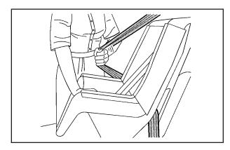
Pull the rest of the shoulder belt all the way out of the retractor to set the lock.
