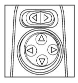
The power mirror controls are located near the driver's window, on the driver's door armrest.
