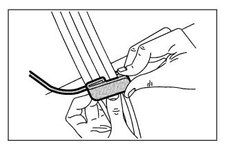
Slide the guide under and past the belt. The elastic cord must be under the belt. Then, place the guide over the belt, and insert the two edges of the belt into the slots of the guide.
