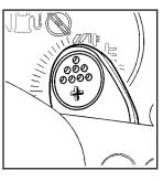
The paddles are located on the steering wheel. They are used to up-shift or down-shift the transaxle.
