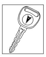
The vehicle is equipped with PASS-Key® III (Personalized Automotive Security System) theft-deterrent system. PASS-Key® III is a passive theft-deterrent system. This means nothing special needs to be done to arm or disarm the system. It works when the key is inserted or removed from the ignition.
