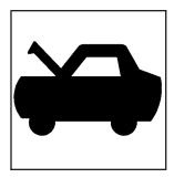
Pull the hood release handle with this symbol on it. It is located inside the vehicle near the parking brake pedal.
