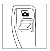
The switch to control the sunroof is located in the headliner.
