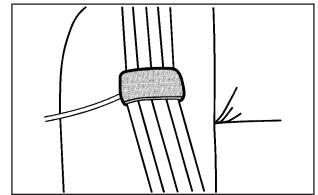
Be sure that the belt is not twisted and it lies flat. The elastic cord must be under the belt and the guide on top.
