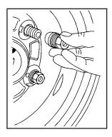
Reinstall the wheel nuts with the rounded end of the nuts toward the wheel. Tighten each nut by hand until the wheel is held against the hub.
