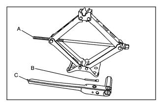
8. The tools you will be using include the jack (A), extension and protector/guide (B) and the wheel wrench (C).
