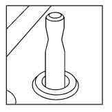
To manually lock or unlock the doors from inside the vehicle, push down or pull up on the door lock pin located on the top of each door panel.
