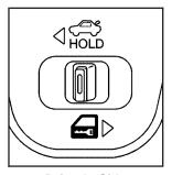
To lock or unlock all doors from inside the vehicle, use the power door lock switch located on either front door.
