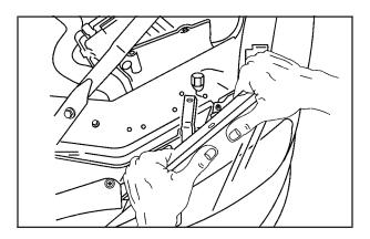
4. Pull the headlamp assembly straight out from the vehicle. (Moving the headlamp up and down slightly may help with its removal.)
