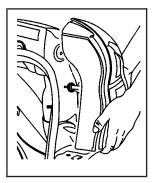
Remove the taillamp assembly by pulling it out from the vehicle.
