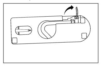
2. Unlock the air compressor hose from the sealant canister by pulling up on the lever.
