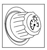
The interior lamps control is located on the instrument panel, to the left of the steering column.
