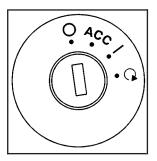
There are four different positions. Insert the key in the ignition and turn it to the right for each position.
