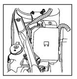
If your vehicle has the 5.3L V8 engine, to uncover the remote positive (+) terminal, remove the fuse block cover.
