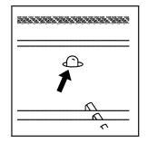
A red light located on top of the instrument panel, toward the center of the vehicle and near the windshield, will flash slowly when the system is armed.
