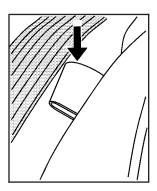
To lower the rear seatback, pull the tab located on the outboard side of the seatback and fold the seatback forward.
