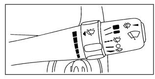
$\heartsuit$  (Windshield Wipers): The lever with this symbol, located on the right side of the steering column, operates the windshield wipers.
