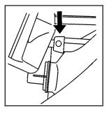
Locate the front turn signal/parking lamp (all models) and fog lamp bulbs (if equipped), which are located below the headlamp assembly.
