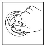
Turn the center nut on the compact spare tire cover counterclockwise to remove it.
