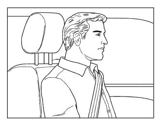
Adjust the head restraint so that the top of the restraint is closest to the top of the occupant's head. This position reduces the chance of a neck injury in a crash.
