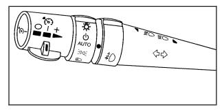
The exterior lamp control is located to the left of the steering wheel on the multifunction lever.
