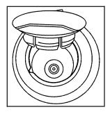
The vehicle has two 12-volt outlets which can be used to plug in electrical equipment.
