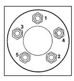
10. Tighten the wheel nuts firmly in a crisscross sequence as shown.
