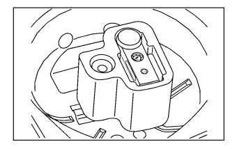
4. Remove the inflator kit by pulling it straight out of the foam container.
