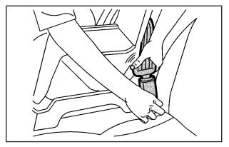
Buckle the belt. Make sure the release button is positioned so you would be able to unbuckle the safety belt quickly if you ever had to.
