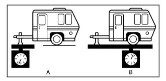
When using a weight-carrying hitch or a weight-distributing hitch, the trailer tongue (A) should weigh 10 to 15 percent of the total loaded trailer weight (B).
