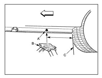
For jacking at the vehicle's rear location, put the jack lift head (B) about 9 inches (23 cm) from the front edge of the rear wheel opening (C). Line up the jack with the arrow (A) as shown.
