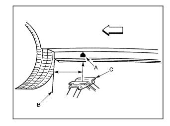
Find the jacking location using the diagram. For jacking at the vehicle's front location, put the jack lift head (C) about 6 inches (15 cm) from the rear edge of the front wheel opening (B). Line up the jack with the arrow (A) as shown.
