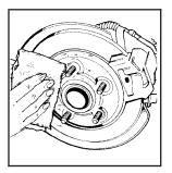
Remove any rust or dirt from the wheel bolts, mounting surfaces and spare wheel. 7. Install the compact spare tire.
