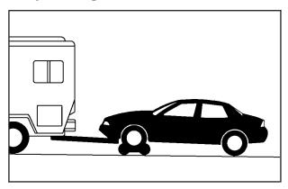
The vehicle can be towed using a dolly. To tow your vehicle using a dolly, follow these steps:
