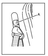
To move it down, pull the release button (A) out and move the height adjuster to the desired position. You can move the height adjuster up just by pushing up on the shoulder belt quide.
