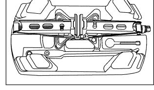
7. Turn the nut holding the jack counterclockwise and remove it. Then remove the jack and wrench.
