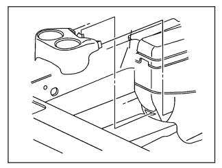
Remove the rear cupholder by pulling it from the console.
