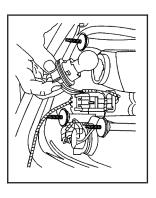
Turn the appropriate lamp socket a quarter turn counterclockwise and remove it.
